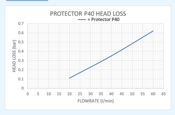
Head loss is calculated with 110µm stainless steel filter and clean water.
