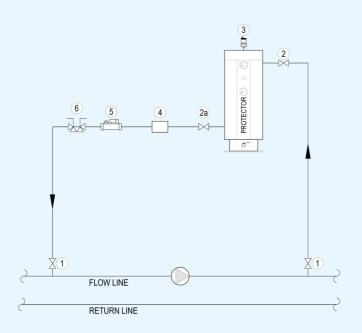
Protector P40 keeps your system clean by adapting to your needs. Two different filtering elements, completely interchangeable, remove suspended particles from the recirculating system.
